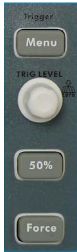
Figure 4-13 Trigger Control Zone
