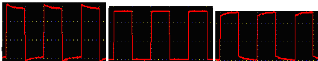
Overcompensated Compensated correctly Under compensated
